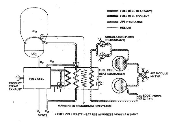
Figure 3-15. Fuel Cell and Heat Exchanger
