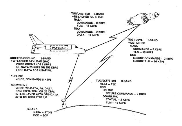
Figure 3-13. Upper Stage Communications Requirements
