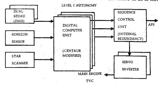
Figure 3-14. Flight Control Subsystem - RLTC
