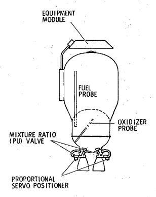
Figure 2-22. PU System Orientation
