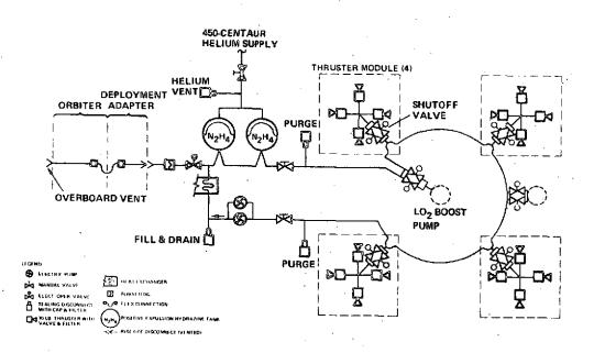
Figure 2-26. Stored Propellants Vented External to Orbiter
