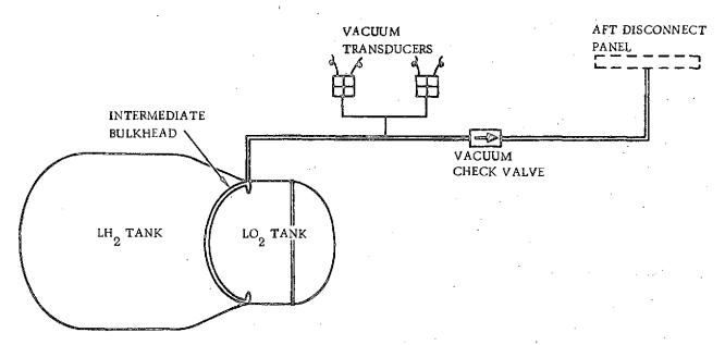
Figure 2-23. Intermediate Bulkhead Vacuum System
