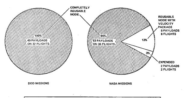
91% OF PAYLOADS CAN BE DELIVERED TO THEIR RESPECTIVE ORBITS IN THE COMPLETELY REUSABLE MODE WITHOUT EXPENDING KICK STAGE OR DROP TANK
