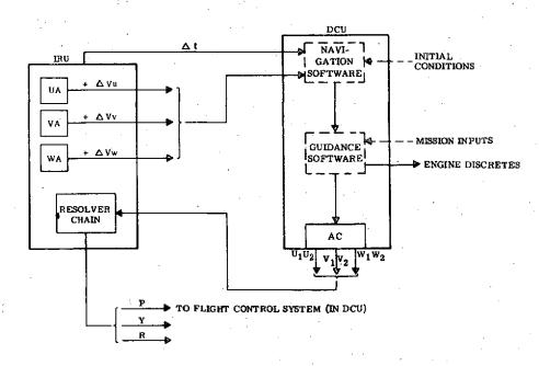
Figure 3-8. Guidance System Block Diagram 3-13
