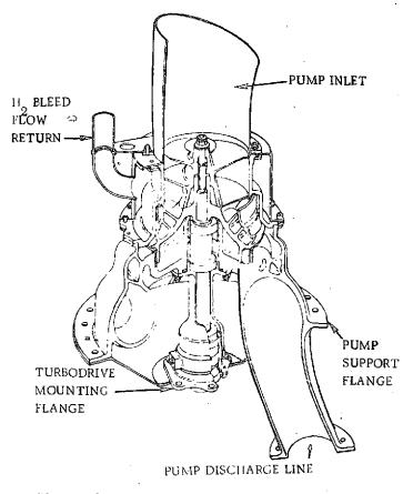
Figure 2-13. Fuel Boost Pump Cutaway
