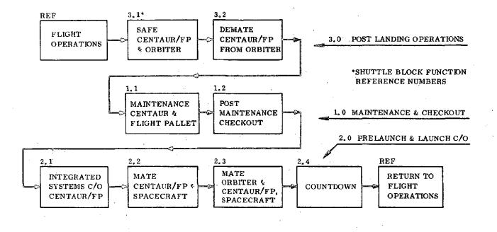
Figure 7-4. Centaur D-1S(R) Top Level Functional Flow Diagram
