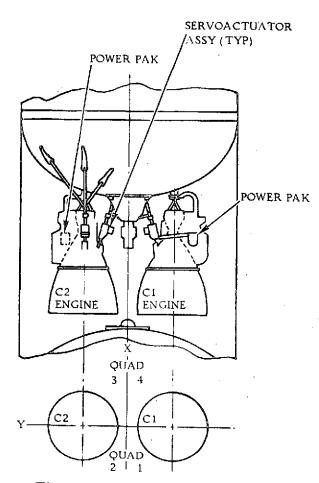
Figure 2-15. Centaur Hydraulic System Orientation
