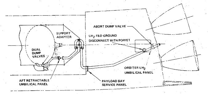
Figure 2-24. LH<sub>2</sub> Fill and Drain System
