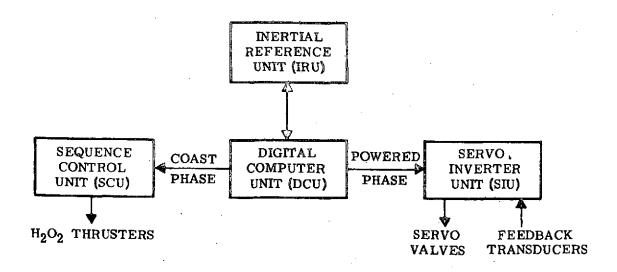
Figure 3-10. Primary Flight Control System
