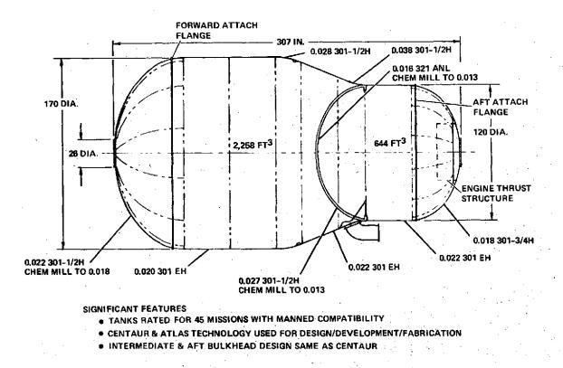
Figure 2-8. RLTC Propellant Tank
