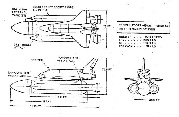
Figure 1-4. Shuttle Vehicle
