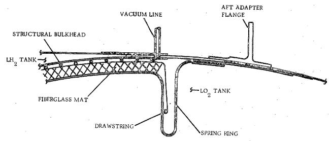
Figure 2-7. Intermediate Bulkhead
