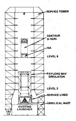
Figure 7-3. Centaur Pre-First-Flight Cryogenic Tanking Test and Checkout Facility. ETR Complex 36
