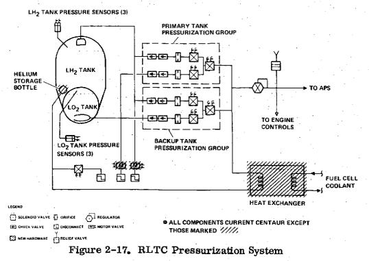
Like D-1S(R) and D-1T, the RLTC  $LH_2$  tank pressurization line terminates in a diffuser and the  $LO_2$  tank pressurization line terminates in a bubbler ring.
