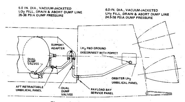
Figure 10-6. LH<sub>2</sub> Fill and Drain System
