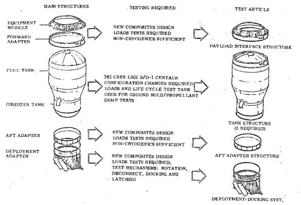
Figure 8-5. Major Structural Tests - RLTC
