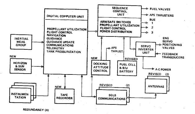
Figure 10-10. Astrionics Functional System
