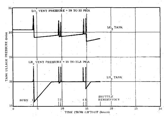
Figure 2-21. D-1S(R) Propellant Tank Ullage Pressure vs Time From Liftoff
