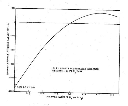
Figure 10-4. Mixture Ratio Effect on Geosynchronous Payload Capability
