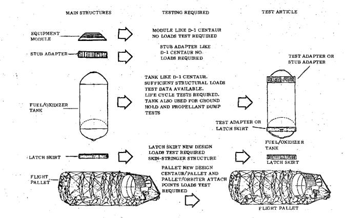
Figure 8-4. Major Structural Tests - D-1S(R)
