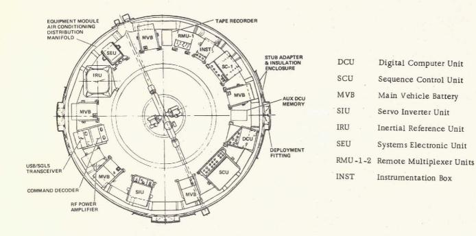
Figure 3-4. Astrionics Equipment Module - D-1S(R)
