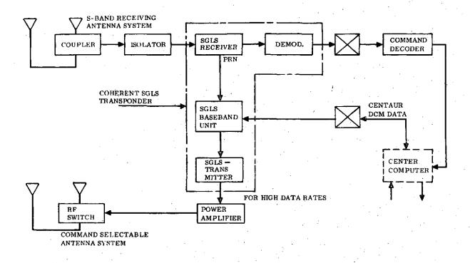
Figure 3-12. Single Channel Functional Diagram - Communications Subsystem (DoD)
