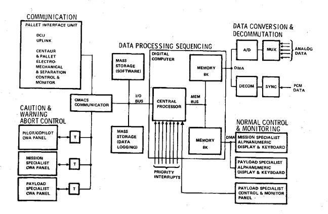
Figure 5-10. CMACS Hardware Block Diagram 5-15
