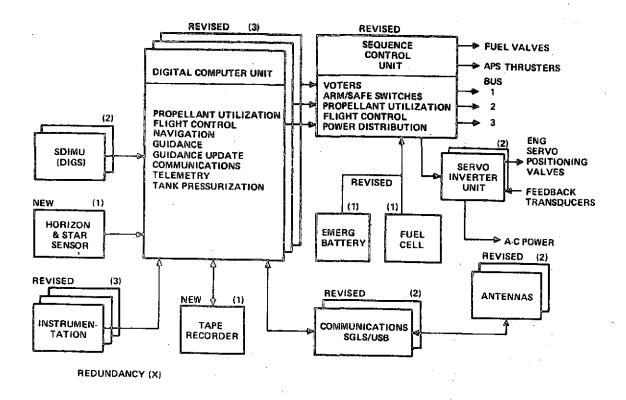
Figure 3-3. Astrionics System - RLTC
