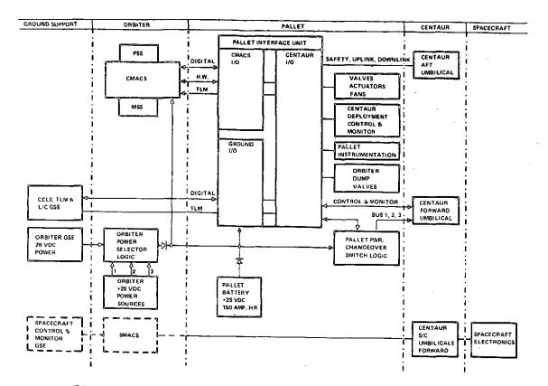
Figure 5-9. Pallet Functional Block Diagram - D-1S(R)
