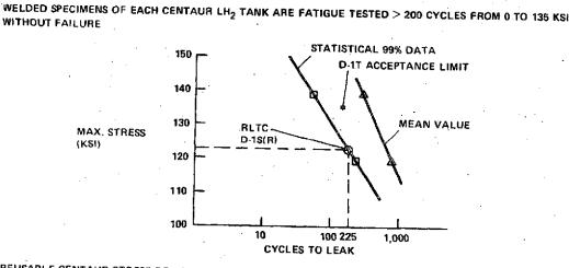
REUSABLE CENTAUR STRESS REDUCED TO 123 KSI FOR MANNED COMPATIBILITY ALLOW FACTOR OF 5 FOR BIAXIAL STRESS, SECONDARY FLUCTUATIONS, ETC.
