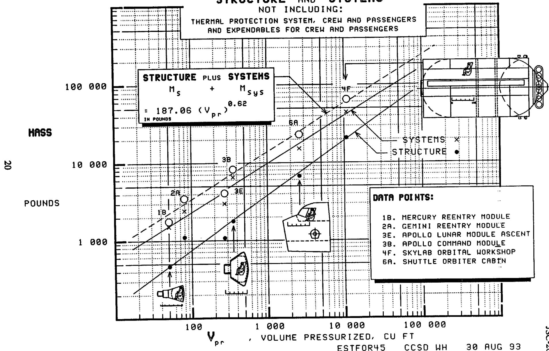
Figure 8 shows a plot of DRY MASS versus wetted area for a number of vehicles, winged and non-winged, but all are manned. Mercury is the smallest hardware value while the Shuttle Orbiter is the largest hardware value. The Shuttle Orbiter has been normalized to the other data by removing the main engines.
