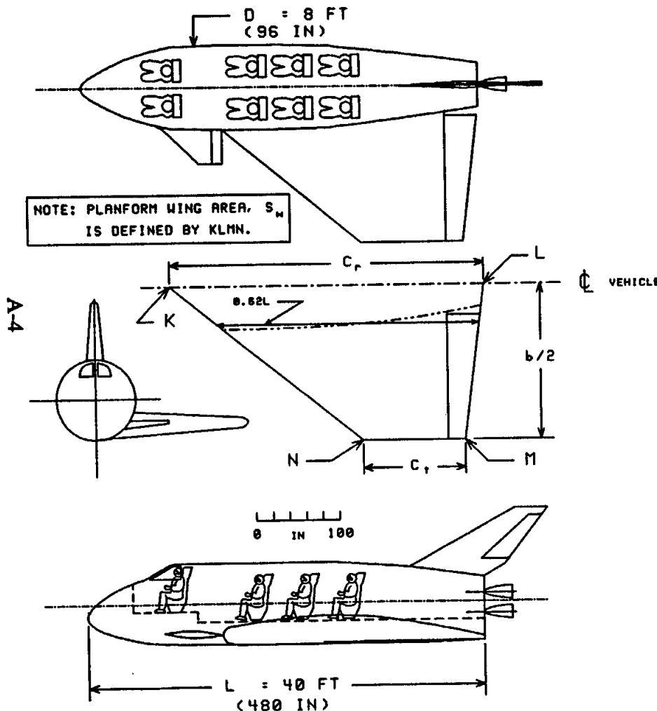
1. BODY WETTED AREA,  $A_b = 0.85(\pi D L) + (\pi D^2/4) = 1,028$  SQ FT, WHERE 0.85 ACCOUNTS FOR THE NARROWING OF THE BODY AT BOTH ENDS, AND  $\pi D^2/4$  ACCOUNTS FOR AN AFT END CLOSURE BASED ON AN AVERAGE D OF 5.4 FT.
