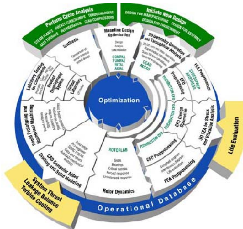
Figure 13 Concepts NREC Turbomachinery Design Process (Used with permission
