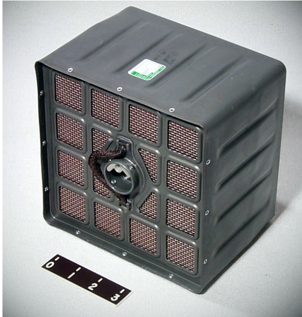
Figure 10: LiOH canisters used by Project Artemis to remove the poisonous \text{CO}_2 gas from the cabin atmosphere.
