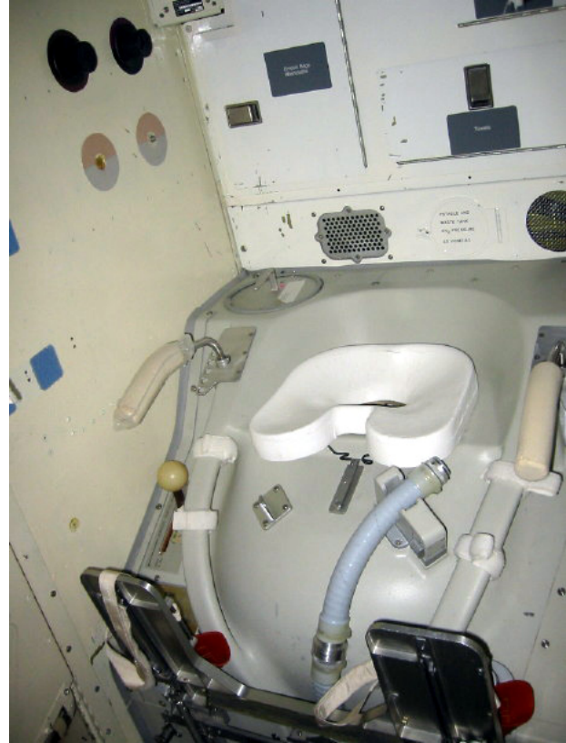
Figure 9: Project Artemis’ toilet system is similar to the one that has been in use on the space shuttle for over two decades.
