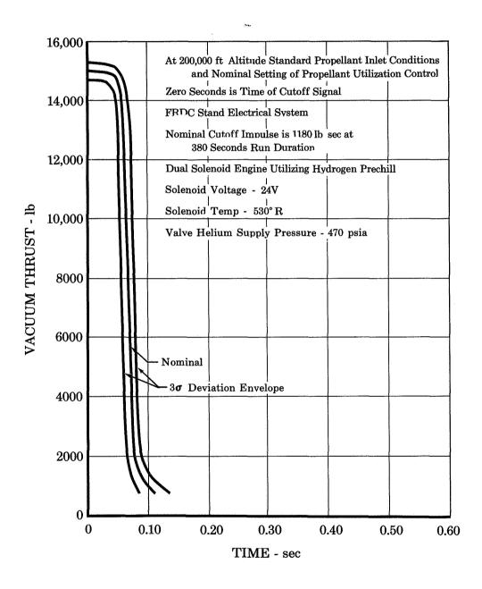
Figure V-3. Estimated Shutdown Transient Thrust vs Time
