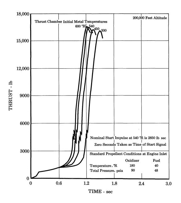
Figure V-2. Estimated Starting Transient Showing FD 8877 Effects of Initial Thrust Chamber Wall Temperatures
