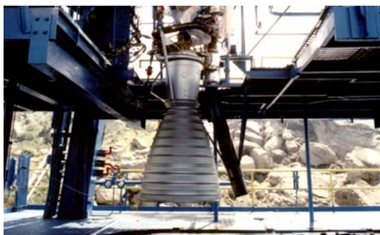
RS-27A engine in place on test stand to be hot fired
