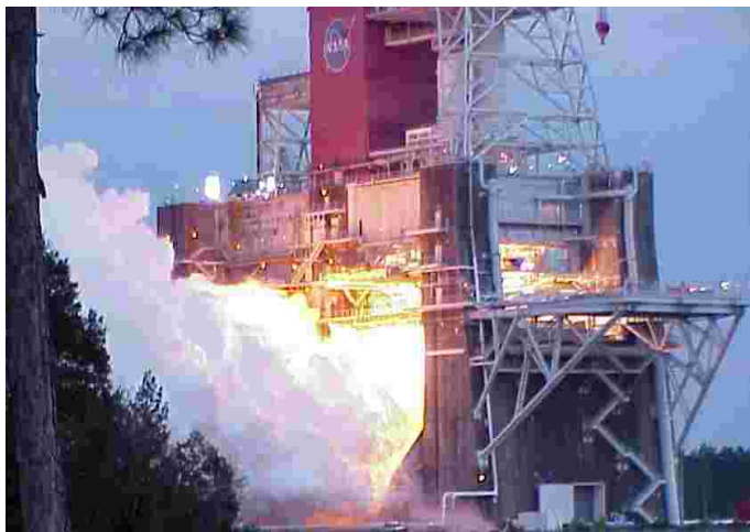
RS-68 hot-fire test at Stennis Space Center, MS
