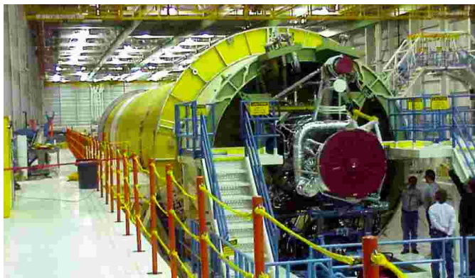
RS-68 mated to Delta IV Common Booster Core, Decatur, AL
