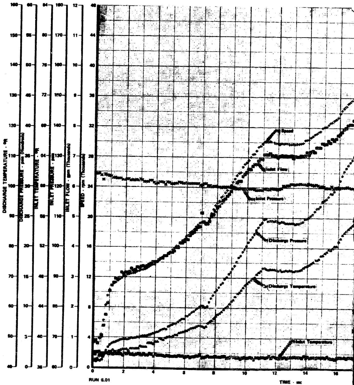
Figure 953. Significant Turbopump Parameters vs Time, Test 6.01, Rig F35155-2, Sheet 1
