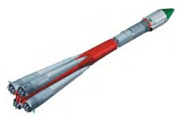
The second stage is similar in construction to the booster stages, using the RD-108A engine and four vernier thrusters for three-axis flight control. The core stage nominally burns for 290 seconds. The stage is shaped to accommodate the boosters, and a stiffening ring is located at the upper interface between the boosters and central core.
