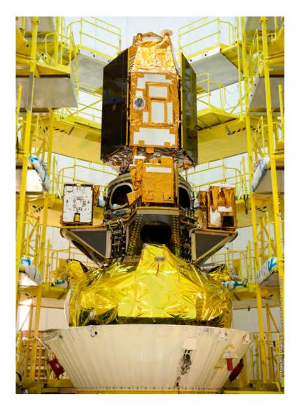
Figure A4c 2-1 Nose block with ASAP-S ready for encapsulation
