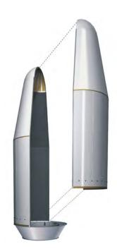
The ST Fairing is  $\emptyset$ 4.11 m in diameter ( $\emptyset$ 3.80 m internal usable volume allocated to the spacecraft) with a length of 11.433 m.
