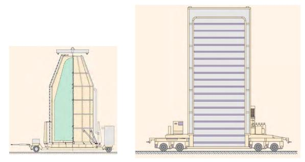
Figure 6.3.4a – The CCU2 and CCU3 payload containers
