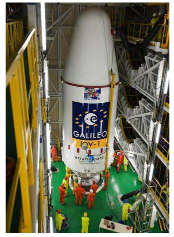
Figure 6.2.3.2.2c – Upper composite hoisting on Launch Vehicle
