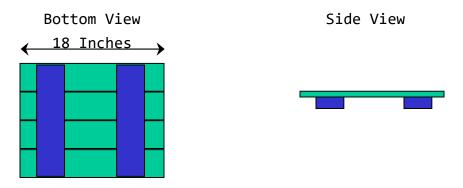
Allow at least 1" clearance When attaching the 2X4's to the bottom so that you can attach the hinge in a later phase
